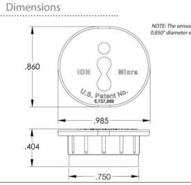
NOTE: The sensor dowel lid has a 0.850" diameter x 0.030" thick.
